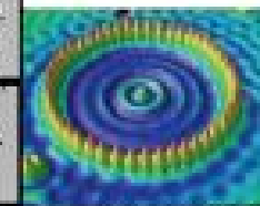
Quantum corral of 48 iron atoms on copper surface positioned one at a time with an STM tip Corral diameter 14 nm
