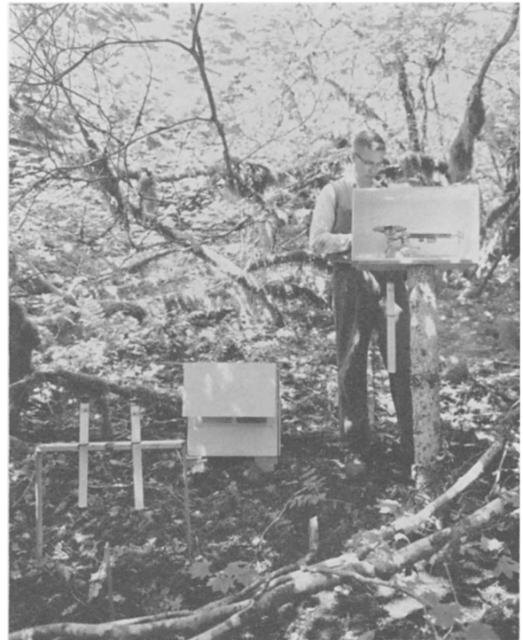
FIG. 3. Balance on weighing platform (right) and rack for holding instruments (left) shown in place in the woods.
