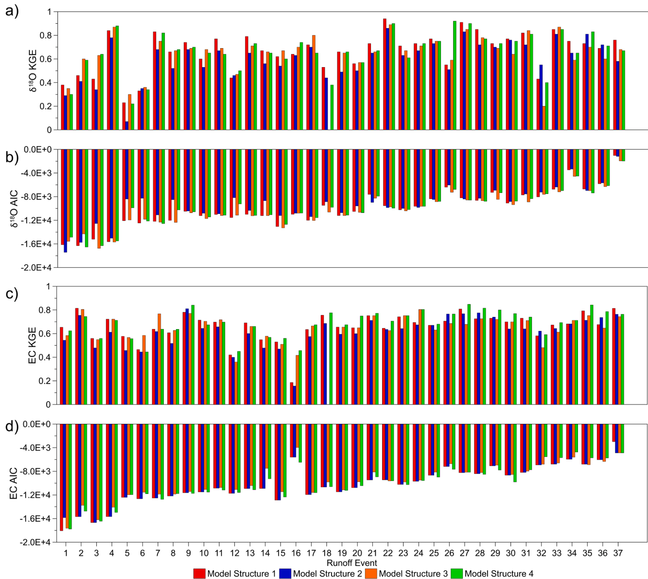
Fig. 3. Best model performance metrics (KGE and AIC) of flow partitioning using high resolution \delta^{18}\text{O} and EC data with each model structure. Red, blue, orange, and green bars correspond to model structures 1, 2, 3, and 4, respectively. Subplots a) and b) correspond to \delta^{18}\text{O} calibration, and (c) and (d) correspond to EC calibration. (For interpretation of the references to colour in this figure legend, the reader is referred to the web version of this article.)
